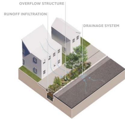
Right-of-way bioswales are vegetated drainage courses located in sidewalks to capture, detain, and infiltrate runoff from streets, allowing any excess rain water to enter the piped stormwater system.
